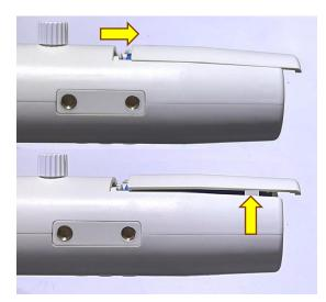
Hold the battery door and slide right to release it first, then lift up to open the battery door.
