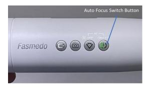
When turn OFF the auto focus, the indicator (the left button of the switch button) will show White light to remind you that the auto focus status is OFF.
