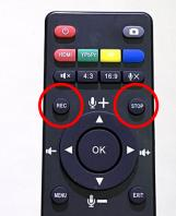
button on the remote controller to start, and push "STOP" button to stop recording.
